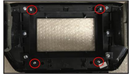
Position the new fascia panel in front of the main air vent/trim panel and screw into place using the screws provided in this kit.
