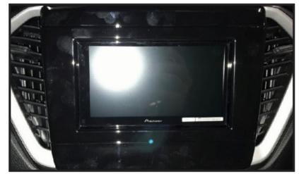
Place the new fascia panel over the front of the new radio to complete the installation.
