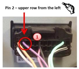
1 Cut the cable at pin 2 of the upper row from the left side and isolate both ends.
