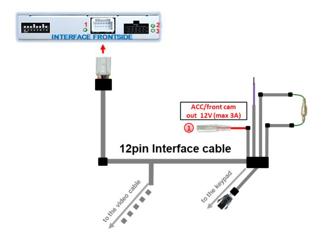
The red power supply output ACC/front cam out 12V (max 3A) can be used to power an external source and has a different assignment depending on the position of dip switch 1 (of the black 8 dips):
