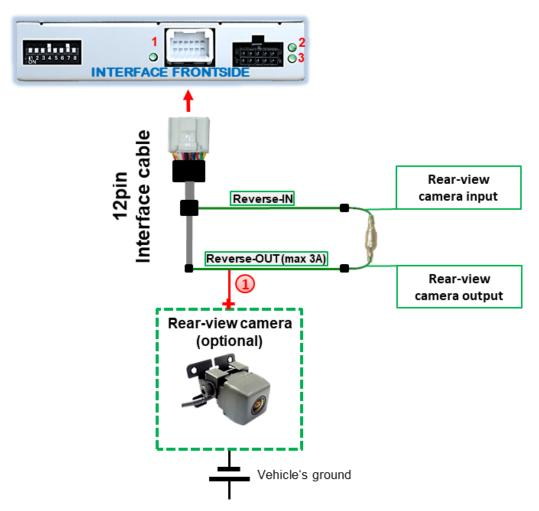
1 The 12 V power supply for the rear-view camera (max 3A) has to be taken from the green wire of the 20pin cable to avoid an unnecessary, permanent power supply to the camera electronic.
