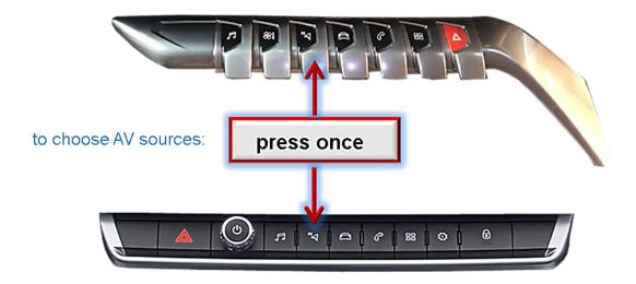
A press of the infotainment's "Navi"-button switches the input from factory mode to the inserted video sources. If, by dip switch setting, all inputs are enabled, the order is the following:
