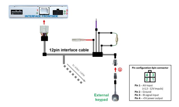
Onnect the keypad's female 4pin connector to the video-interface's male 4pin connector.
