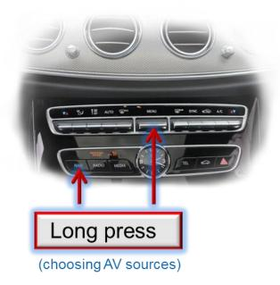
A long press of the NAVI button or the Menu button switches the input from factory mode to the inserted video sources.
