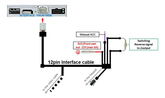
1 The red power supply output ACC/front cam out 12V (max 3A) can be used to power an external source and has a different assignment depending on the position of dip switch 1 (of the black 8 dips):
