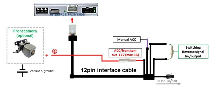
1 The red power supply output ACC/front cam out 12V (max 3A) can be used to power a front camera. If Dip 1 is set to ON (of the black 8 dips), the power supply output gives +12V (max 3A) when reverse gear is engaged plus 10 seconds delay after reverse gear is disengaged.
