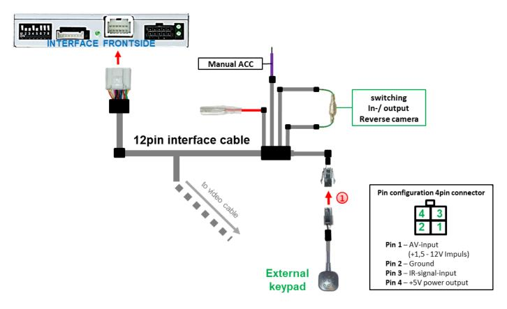
Onnect the female 4pin connector of the keypad to the male 4pin connector of the 12pin interface cable.
