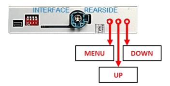
The picture settings are adjustable by the 3 push-buttons on the video-interface. Press the MENU button to open the OSD settings menu or to switch to the next menu item. Press UP and DOWN to change the selected value. The buttons are placed inside in the housing to avoid accidental changes during or after the installation. Picture settings must be done separately for Video1, Video 2 and rear-view camera while the corresponding input is selected and visible on the monitor.
