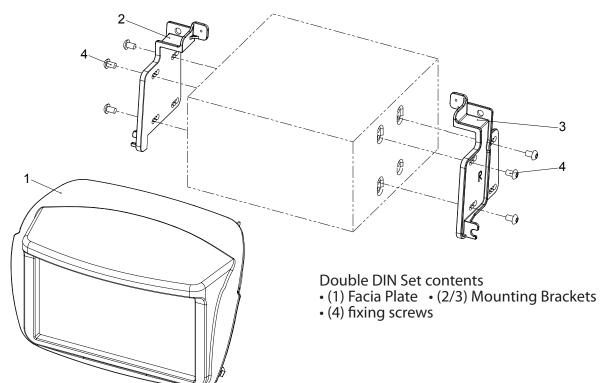
Attach mounting brackets left (L) and right (R) to Pioneer Navigation (use the first of three possible holes as shown on the photo below)
