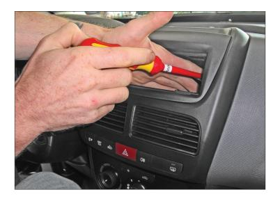
2. Remove 2 screws (left and right)
