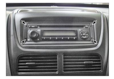
1. Remove OEM Radio with special radio release keys
