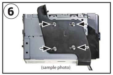
Mount the left and right brackets to the head unit using the supplied hex screws. Please see Diagram on Page 4 for instruction on how to fit a Single DIN unit with pocket instead of a Double DIN unit as shown in the image.
