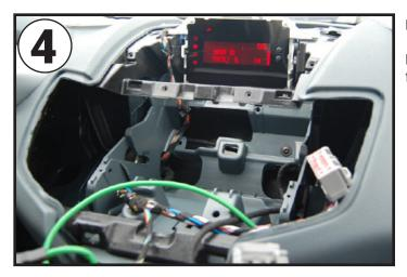
Remove the OEM head unit and disconnect all wiring
