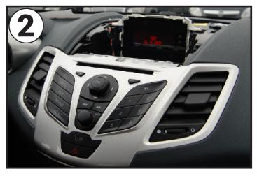
Remove the entire trim panel and place safely to one side for reassembly
