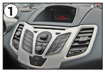
Use a panel removal tool to unclip the panel surrounding the small dash display
