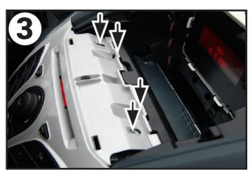
Remove the four screws highlighted by the arrows located above the OEM head unit
