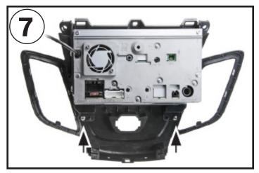
Mount the head unit to the fascia panel using the supplied Phillips screws at the points highlighted by the arrows in the image.
