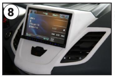
Make all required wiring connections to the back of the aftermarket head unit and fit the head unit/fascia assembly into the dashboard cavity to complete the installation.
