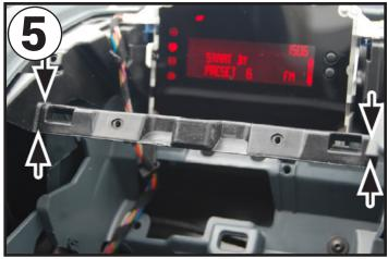
Use a cutting tool to remove the middle bar (highlighted by the arrows in the image) to allow space for the new head unit to fit into the dashboard cavity.
