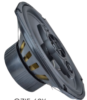
GZIF 69X High quality 3-way coaxial speaker 120 WRMS / 180 WMAX Freq. response 40 – 20000 Hz 13 mm / 0.51" Mylar tweeter 50 mm / 2" Mylar midrange
